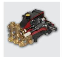
The U-Seals provide better run-dry protection, extend pump life, and allow for inlet water of up to 145°F. Kärcher K3 pumps provide a stronger crankcase with thicker mounting feet and extra-large European made tapered roller bearings for longer pump life. The crankcase is reinforced and comes with the new O-ring seal for leak-free operation. Specially die cast connecting rods provide for quieter operation and longer pump life.
