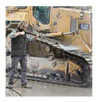
The Kärcher dirt-blaster combines the advantages of pencil jets and fan jets. The nozzle spins at approximately 4,000 rpm to apply a powerful cleaning spray to a large area.
