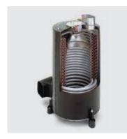
Kärcher's proprietary heating coil is unequaled in the industry for its high heating performance, compact design, and super-efficiency. Double-wall construction – with air passing between the two walls – provides insulation as well as oxygen for the combustion process.
