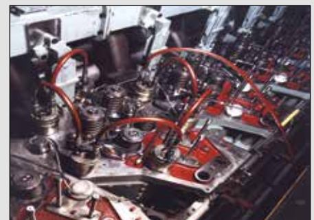
▲ Hydraulic nuts on a diesel engine.
