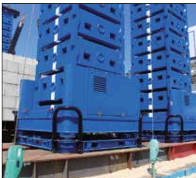
▼ Enerpac has been awarded a contract by Burkhalter to extend the height of Enerpac's 2000 ton (500 ton per tower) jack-up system from 20m to 36m for future projects.
